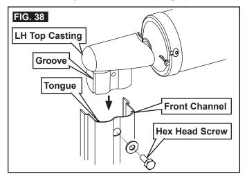
2. Reinstall hex head screw (and washer) to secure front channel to top casting. See (FIG. 38).
