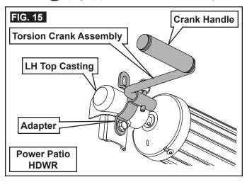
5. AWARNING IMPACT OR PINCH HAZARD. Do NOT remove cotter pin from torsion rod (at end cap) until top casting is securely held. Otherwise, rapid casting spin off will occur. Spring tension will attempt to spin the top casting and/or fabric roller tube quickly and unexpectedly. Failure to obey this warning could result in death or serious injury.
