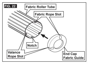
2. Insert fabric rope and valance rope of awning fabric into corresponding slots on fabric roller tube (through end cap fabric guide). See (FIG. 23).
