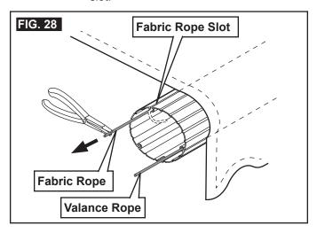
3. Trim fabric rope length according to the appropriate procedure.
