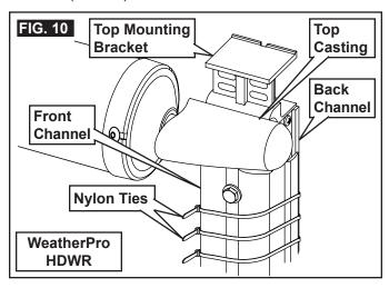
5. Wrap at least (1) nylon tie around front and back channel near bottom of arm assembly, and tape in place. See (FIG. 11).
