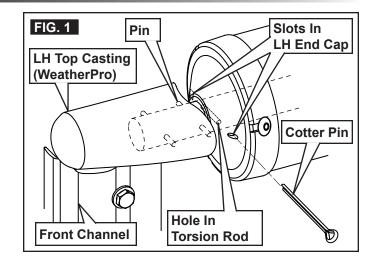
Insert a 7/64" X 2-3/4" cotter pin through end cap and torsion rod. Then tape head of cotter pin to end cap to secure in place. See (FIG. 1).
