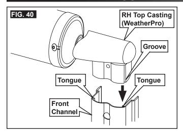
2. A WARNING IMPACT OR CRUSH HAZARD. Make sure top casting is aligned and seated correctly into front channel. Otherwise, top casting could move unpredictably and become unstable, causing awning to [detach / bend / collapse]. Insert RH top casting into front channel until seated securely. See (FIG. 40).
