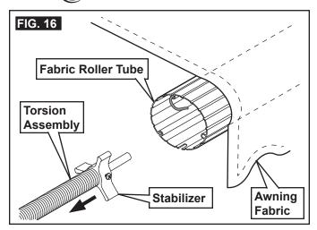
3. Remove burrs, and discard any rivet bodies and debris from fabric roller tube. See (FIG. 16).
